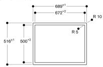
measurements in mm
