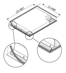
2 The front and rear pegs are reinforced underneath. The strut width is determined by the producer of the stone worktop. The minimum peg width can vary according to the properties of the stone.
