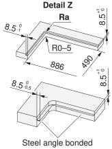
The front and rear pegs are reinforced underneath. The strut width is determined by the producer of the stone worktop. The minimum peg width can vary according to the properties of the stone.
